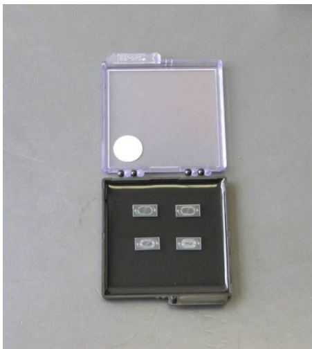
This figure shows four silicon-Pyrex wafers with 40, 60, 80, and 100 mm length microchannels, respectively.
