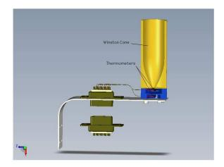
Cut-away drawing of the radiometer, electrical connector, and bracket. The length of the radiometer in this version is about 50 mm. Note the two thermometers (black) in the lower portion. For ease of drawing the upper portion of the Winston cone is shown as cylindrical rather than parabolic.
