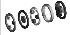
By incorporating helical gear teeth forms (including herringbone), gear bearings provide outstanding thrust bearing performance. They also provide unprecedented high- and low-speed reduction through the incorporation of phase tuning. Phase tuning allows differentiation in the number of teeth that must be engaged
