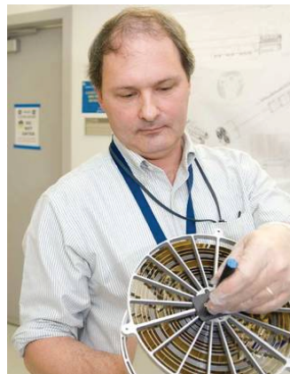
Keith Gendreau holds an assembly of X-ray focusing mirrors similar to those used on NICER/SEXTANT missions. Photo Credit: Bill Hrybyk/NASA
