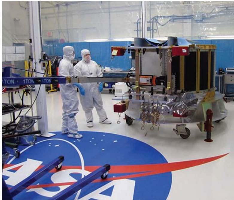
Here, critical welds are X-rayed on the MMS fluid transfer system. —PHOTO BY NASA
